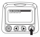
5. The "Use Defaults" screen will be displayed during the resetting period then will automatically return to the "Setup 4- Up Display" menu.
